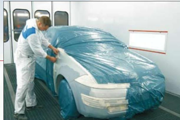
Lacquers and coatings are essential for the protection and esthetics of all kinds of vehicles. Upon assembly, as well as in the after market, the application of new lacquers is a precise and important process. Under the trade name 'Hytiprotect', Hyplast offers a range of high-quality masking films. Next to the standard range, Hyplast offers a product line for large vehicles, as jeeps and small trucks, and a special range for high temperature applications like infrared drying.
